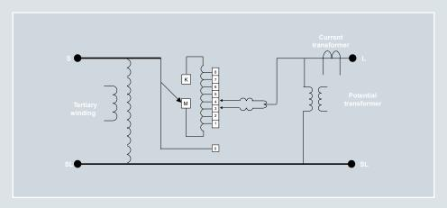
An auto-transformer is a transformer in which primary and secondary windings are coupled both magnetically and electrically as seen above. An input of 100 V will be stepped up to 110 V if the secondary winding is connected in to the high side of the primary winding in series. This is a step-up auto-transformer. When the other end of the secondary winding is connected to the primary winding in reverse polarity, the output will read 90 V for an input of 100 V. This is a step-down auto-transformer.
